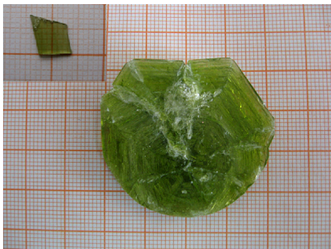
Fig. 2. Photograph of the grown \text{Cr}^{3+}:\text{CsAl}(\text{MoO}_4)_2 crystal.
